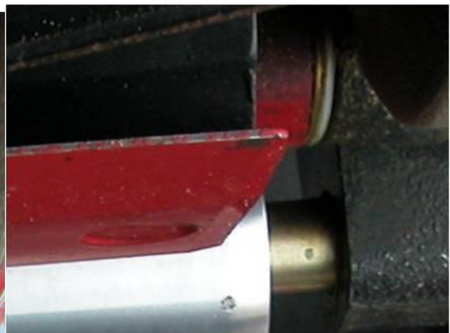
A new bedknife installed on the same mower.
