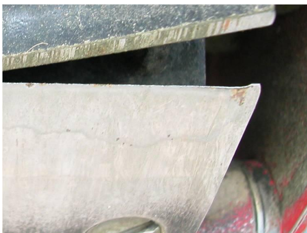
A worn bedknife that needs to be replaced.
